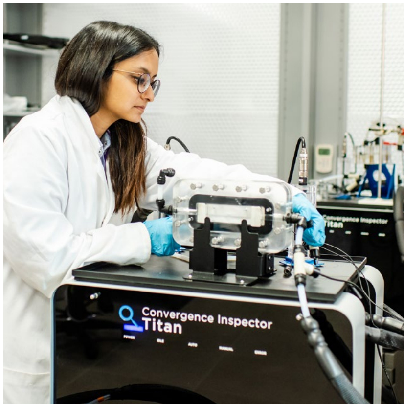
State-of-the-art membrane-based desalination systems: the image shows a researcher working on a membrane distillation unit for desalting highly saline waters to produce fresh water.
