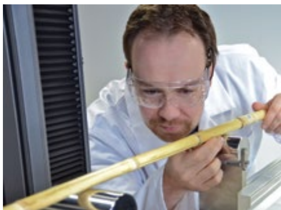
Douglas Cook, assistant professor of Engineering at NYU Abu Dhabi, is using x-ray CT scans and mechanical tests to measure the geometry and material properties of corn stalks in an effort to discover how the corn stalk can be modified to prevent stalk collapse.
