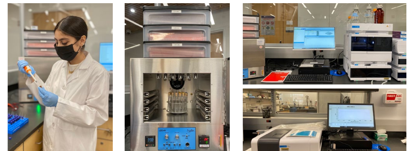
Experimental set up for direct photodegradation and molar absorptivity measurements
