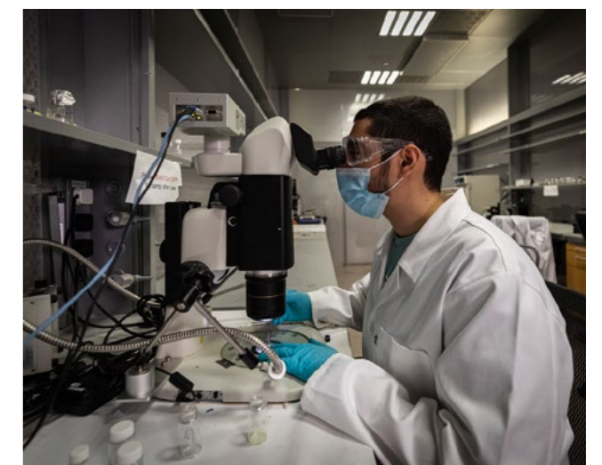
Khalifa Almheiri's quality assessment of (soft actuators/ smart materials) using an optical microscope
