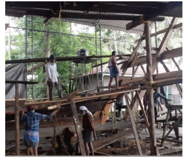
Boatbuilders at Beypore work together to build a baghlah
