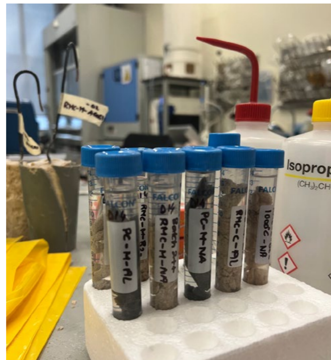
Sample fragments in isopropanol to stop hydration
