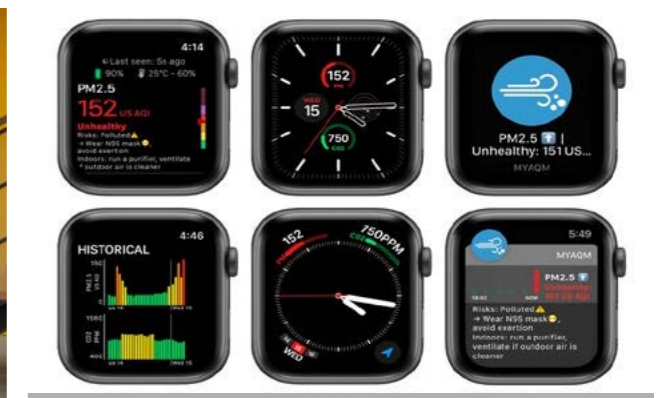
The Apple Watch app interfaces developed by Vince to visualize air quality data fetched from the portable air quality monitor
