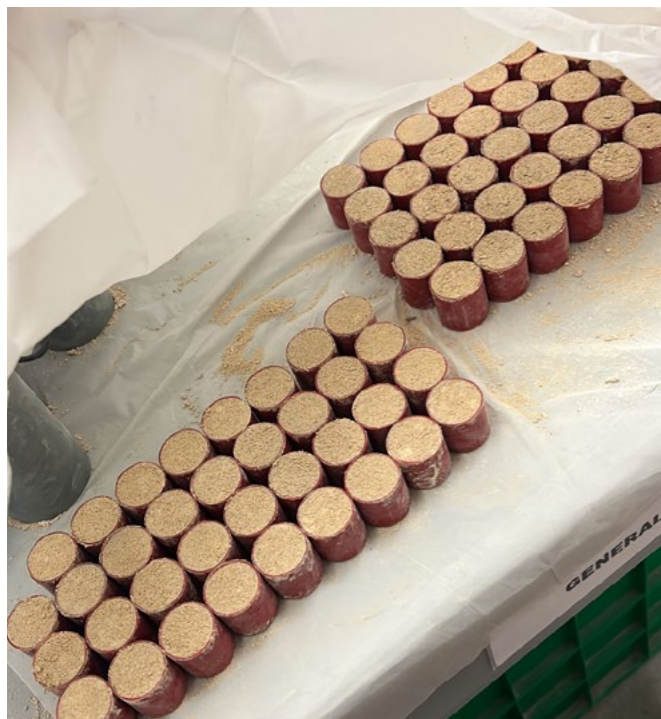
Samples cast in molds for compression testing
